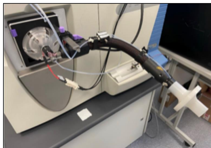
Image 1: Experimental Set-up of the SICRIT Breath Analysis Module in Diluted Breath Mode.
